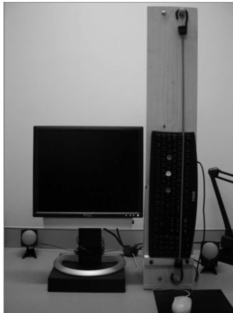
Fig. 1. Apparatus setup. The keyboard was strapped onto a wooden board apparatus with a bungee cord. The end of the keyboard with the “Q” key was positioned at the top, and the end with the “P” key at the bottom. In this setup, the computer screen was raised or lowered to match the participant’s eye level. The height of the keyboard was also adjusted for each participant to ensure that the white home key (“H” key) was aligned horizontally with stimulus presentation on the screen.
